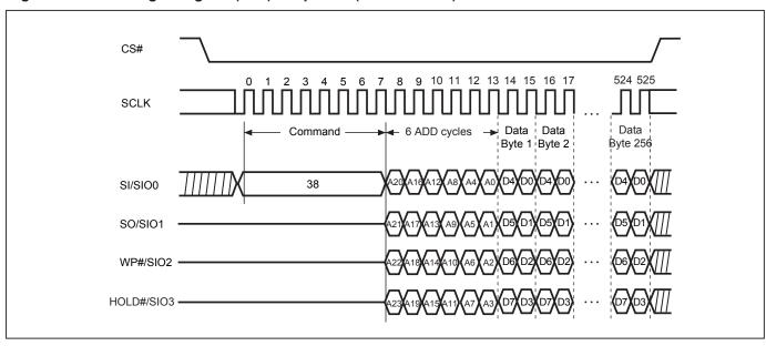
Figure 31. Continously Program (CP) Mode Sequence with Hardware Detection (Command AD)
