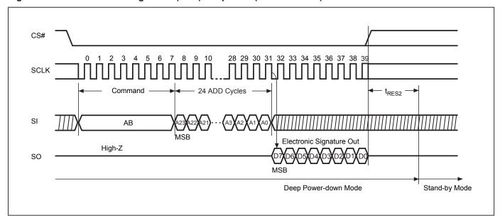
Figure 35. Release from Deep Power-down (RDP) Sequence (Command AB)
