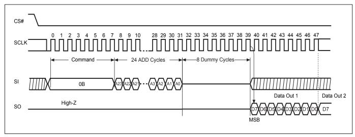
Figure 19. Fast DT Read (FASTDTRD) Sequence (Command 0D)
