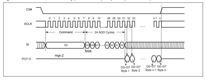
Figure 32-7. Parallel Mode Page Program (Parallel PP) Sequence (Command 02)
