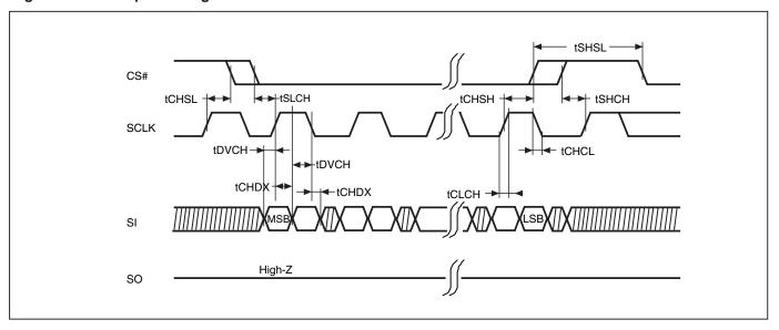
Figure 9. Serial Output Timing for Double Transfer Rate Mode
