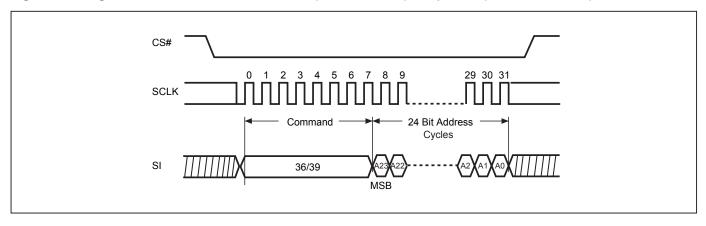
Figure 39. Read Block Protection Lock Status (RDBLOCK) Sequence (Command 3C)
