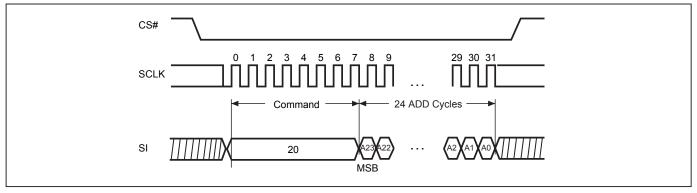
Figure 27. Block Erase (BE/EB32K) Sequence (Command D8/52)
