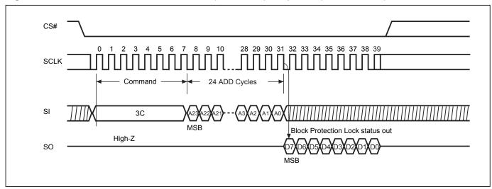
Figure 40. Gang Block Lock/Unlock (GBLK/GBULK) Sequence (Command 7E/98)
