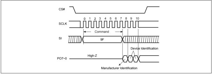
1. There are 3 data bytes which would be output sequentially for Manufacturer and Device ID 1'st byte (Memory Type) and Device ID 2'nd byte (Memory Density).
