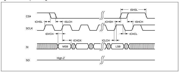
Figure 7. Output Timing
