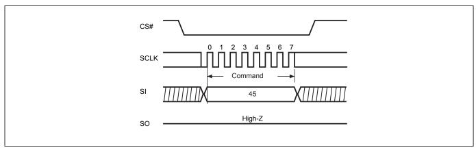
Figure 32-3. Parallel Mode Read Identification (Parallel RDID) Sequence (Command 9F)
