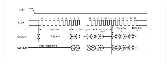
1. SI/SIO0 or SO/SIO1 should be kept "0h" or "Fh" in the first two dummy cycles. In other words, P2=P0 or P3=P1 is necessary.
