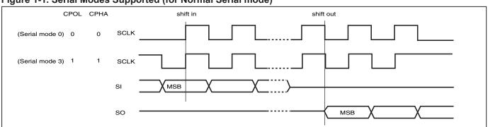
Figure 1-1. Serial Modes Supported (for Normal Serial mode)
