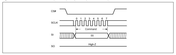
Figure 32-2. Exit Parallel Mode (EXPLM) Sequence (Command 45)
